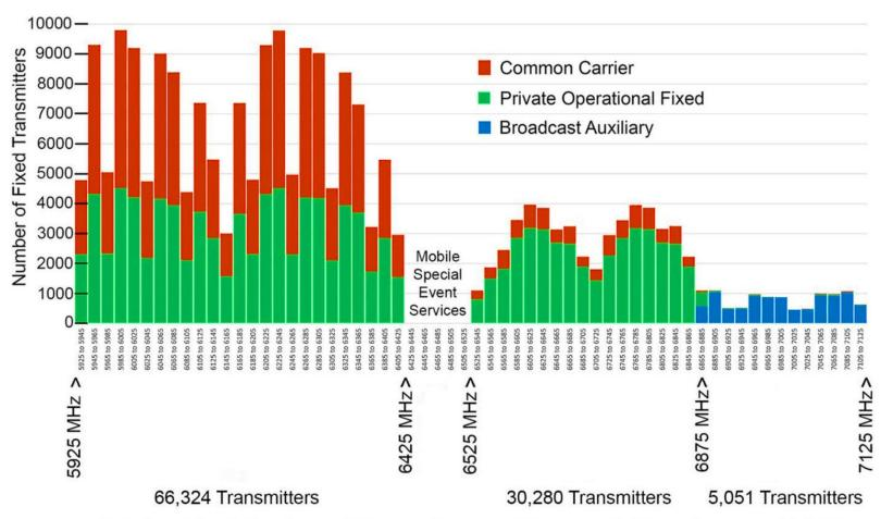
Existing Fixed Co-channel Transmitters and Proposed Allocations per 20 MHz data and graph provided by Comsearch
