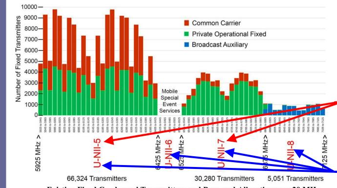
Existing Fixed Co-channel Transmitters and Proposed Allocations per 20 MHz data and graph provided by Comsearch
